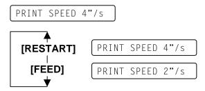
After selecting the print speed, press the **[PAUSE]** key to go to Sensor Type Selection.
